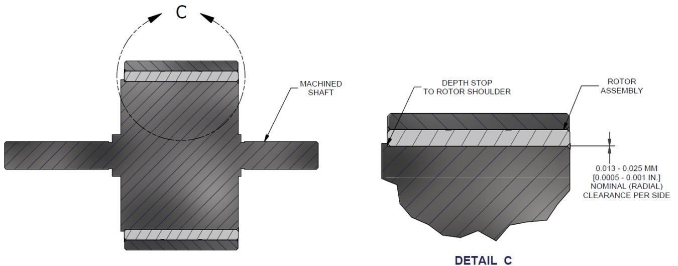
Figure 7. Detail view of Rotor Shaft Assembly
