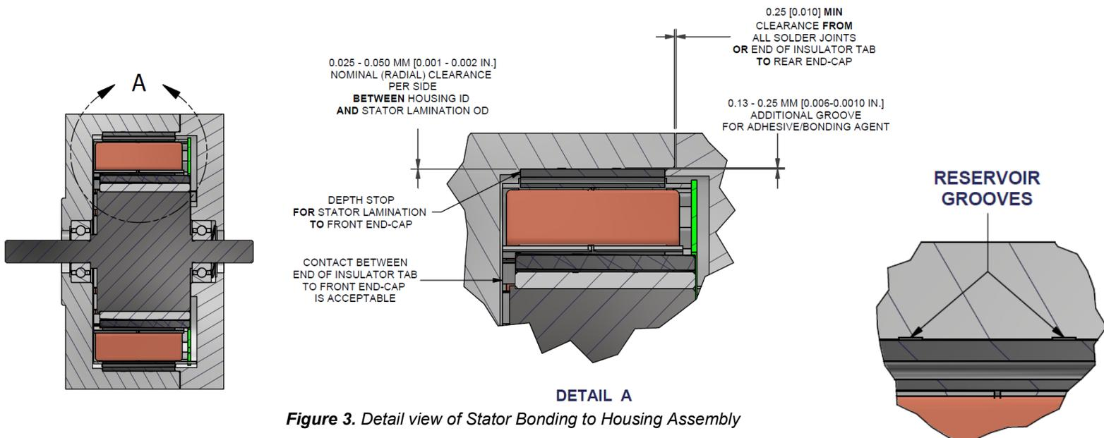
**Figure 3. Detail view of Stator Bonding to Housing Assembly**
